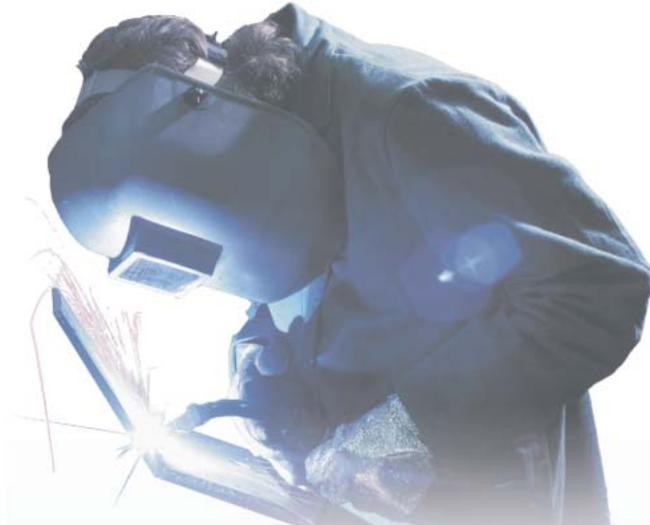
The secret is getting rid of the oil. Burning through the oil film generates additional contaminants and gives a less uniform weld bead that serves to weaken the weld. Welds of SCS plates have been shown to be 20% stronger than comparable welds of P&O. And SCS' more uniform weld bead reduces filler wire consumption by up to 30%.
