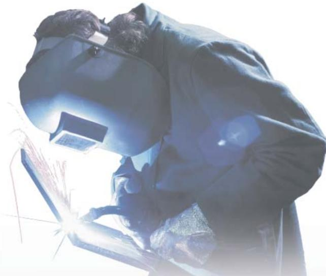
The secret is getting rid of the oil. Burning through the oil film generates additional contaminants and gives a less uniform weld bead that serves to weaken the weld. Welds of SCS plates have been shown to be 20% stronger than comparable welds of P&O. And SCS' more uniform weld bead reduces filler wire consumption by up to 30%.
